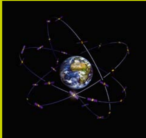
The Galileo constellation provides global coverage through 27 operational and 3 in-orbit spare satellites in 3 orbital planes. Image: ESA
