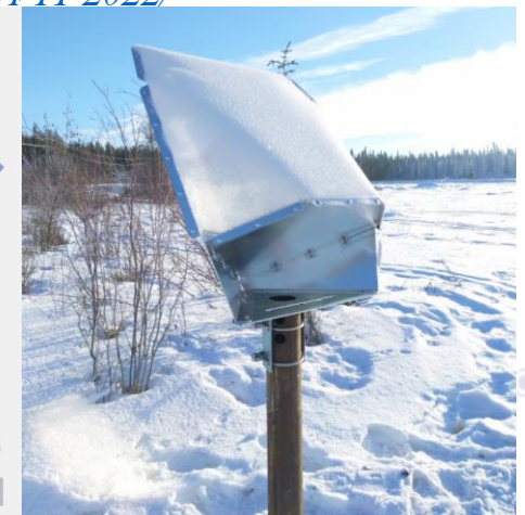
Corner reflectors – a solution to vegetation, changing texture Image attribution: Tre Altamira
