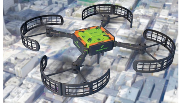
TRIUMPH-F1 is equipped with four-angled documentation cameras and a downward high-precision camera for photogrammetry
