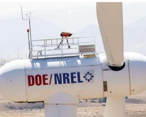
Wind Iris nacelle-mounted LiDAR from Avent Lidar Technology and Renewable NRG Systems
