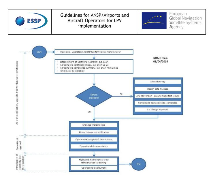
Figure 7-1 Overall process of the LPV capability implementation
