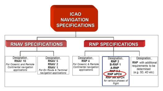
Figure 3-1 Navigation Specification according to the PBN Manual
