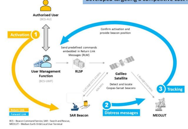
SAR/Galileo Beacon Command Service High-Level Concept for Remote Beacon Activation
