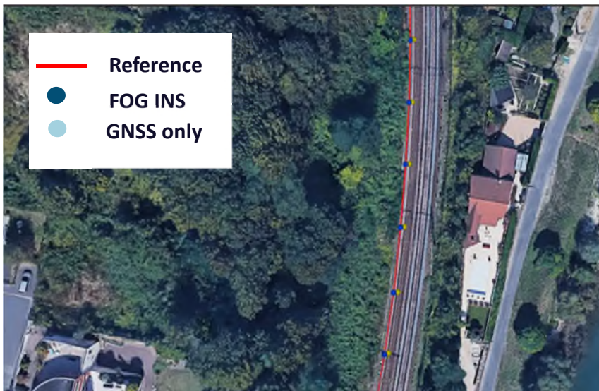
Figure 3-2 – Illustration of localisation test result done by the SNCF using INS sensor
