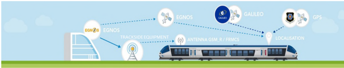
Figure 1-1 – High-level architecture of the train localization system considered in the EGNSS-R project
